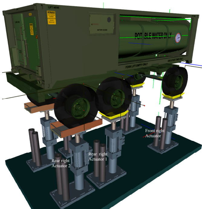
Figure 2 Instrumented PLS (Palletized Load System) tanker-trailer mounted on an n-post motion simulator that was used to validate the present finite element model.
