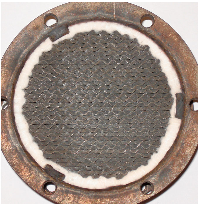
Figure 10: Setup of the permeable cross corrugated substrate (example: foam catalyst)
