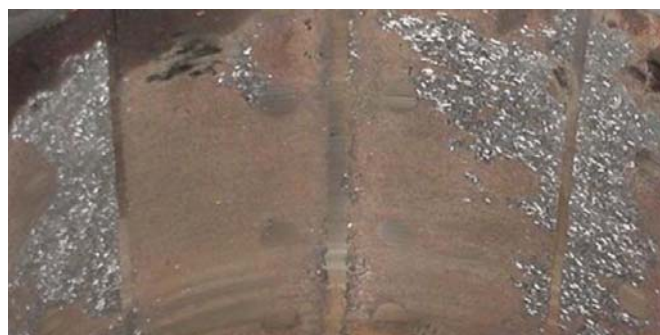
Figure 1. The residual lining was visible on the drum surface after the lining was broken free using external forces
