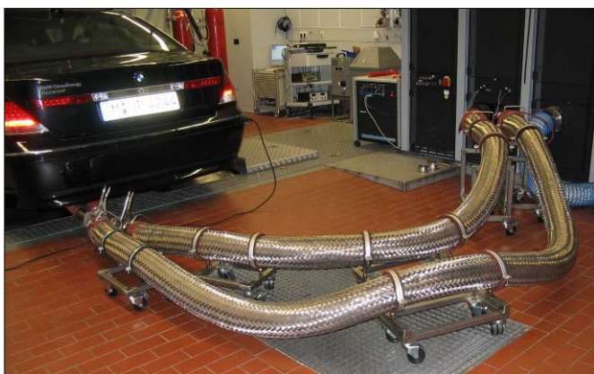
Figure 3: Heated connection tailpipe to CVS
