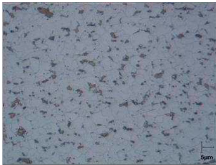
Figure 1. Final microstructure of Ductibor 500P at 30°C/sec (Die-quench). Ferrite + Martensite < 10%
