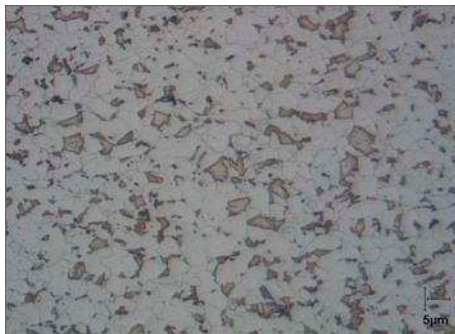
Figure 2. Final microstructure of Ductibor 500P at 100°C/sec (Water-quench). Ferrite + Martensite 10% to 20%
