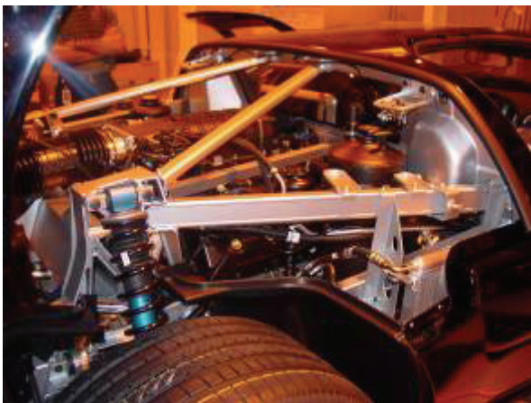
Figure 10: Ford GT Spaceframe extrusions
