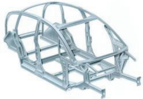
Figure 5: Audi A2 is using many hydroform parts in its aluminum space frame structure (Courtesy of Audi)
