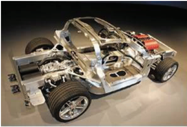
Figure 8: Chevrolet Corvette Spaceframe [4] (Courtesy of GM)
