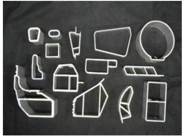
Figure 11: Ford GT spaceframe extrusion cross-sections
