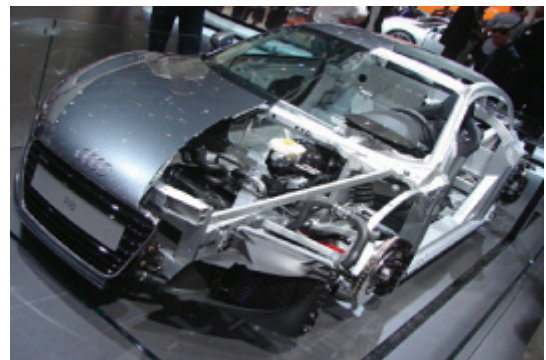
Figure 6: Spaceframe Architecture of Audi R-8 [3] (Courtesy of Audi)
