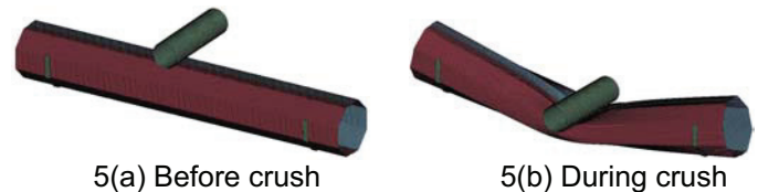
Figure 5. FEA bending crush model
