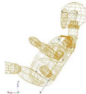
Figure 14: Locations and orientations of accelerometers on forward facing Q1.5 Dummy Model. The Q3 has accelerometers in similar locations.
