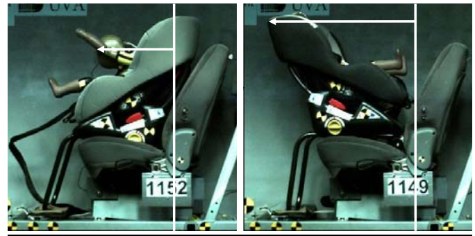
Figure 13: X-Excursions as defined for the model validation. FFCRS excursion was measured from the LATCH bars to the forward-most point of the head. RFCRS excursion was measured from the LATCH bars to the forward-most point of the CRS
