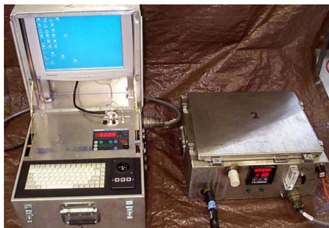
Figure 3 WVU MEMS data collection (left) and emissions sampling box (right).
