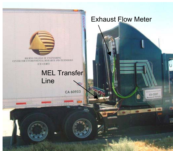
Figure 1: Exhaust flow meter location and MEL sample transfer line
