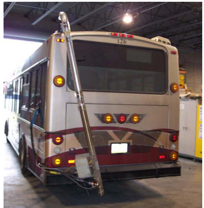
Figure 2. MEMS Exhaust Flow Rate Measurement System Installed on a Test Vehicle
