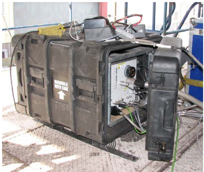
Figure 1. The Horiba OBS-2200 PEMS Installed on a Haul Truck
