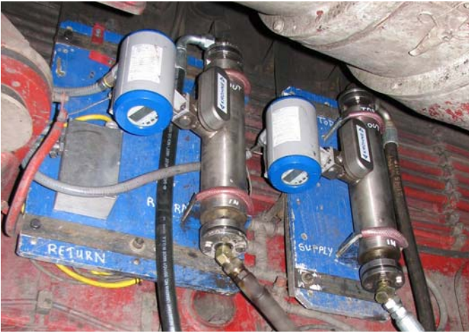
Figure 2. Truck-Mounted Krohne Coriolis Mass Flow Meters
