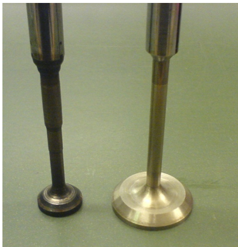
Figure 2 Picture illustrating the difference between the “small tank valve” and the “large tank valve”
