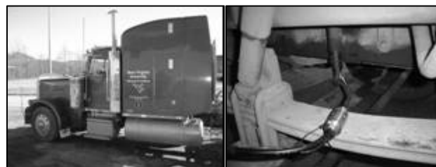
Figure 8: 1996 Peterbilt tractor truck and the sampling port
