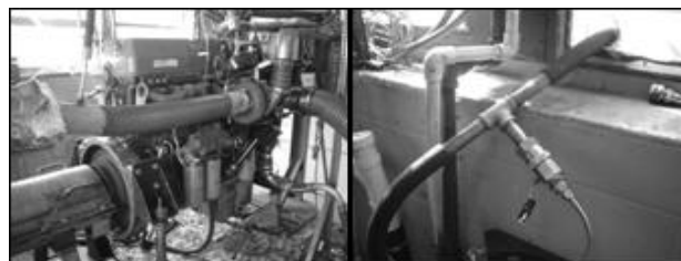
Figure 1: 1992 DDC Series 60 engine and the sampling port (The crankcase was vented through the 1 inch nominal diameter pipe and the sample was collected through the T junction.)
