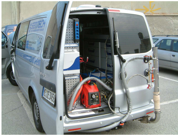
Figure 4: Picture of PEMS installation on board of the VW T5, 2.5 litre van for on road measurements.
