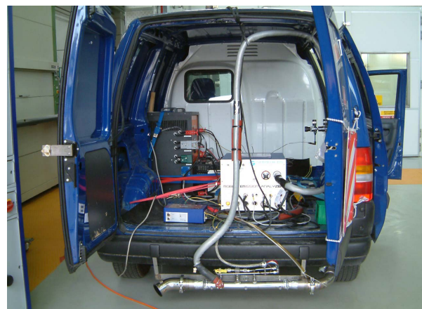
Figure 3: Picture of PEMS installation on board of the 2 litre Fiat Scudo Diesel; the same set-up was used for chassis dynamometer testing in the test cell.
