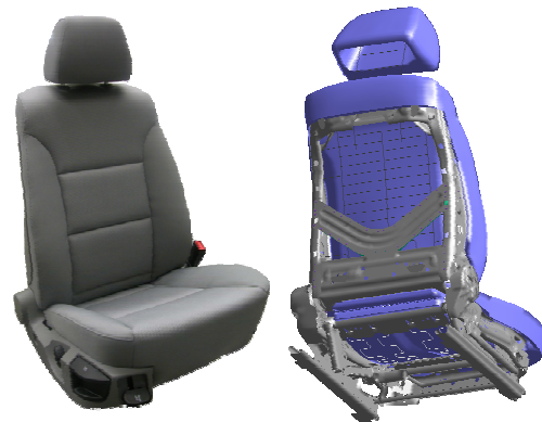
Fig.1: BMW vehicle seat (left) and finite element model (right)
