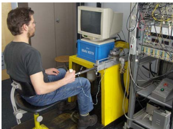
Figure 3. The Proprio manipulator. The subject was seated in a chair while holding the handle of a hydraulic actuator. The subject was positioned in such a way that the elbow made an angle of 90 degrees of flexion. Force perturbation applied through the handle resulted in ante/retroflexion movements of the shoulder joint. To prevent drift and to motivate the subject the actual position of the handle was shown on the display.
