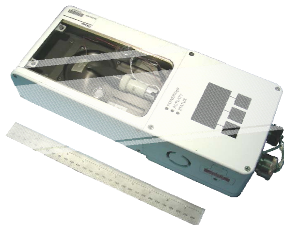
Figure 1: The Third Generation ENose. The Sensor Unit is enclosed in the Interface Unit, which will be connected to the ISS EXPRESS Rack
