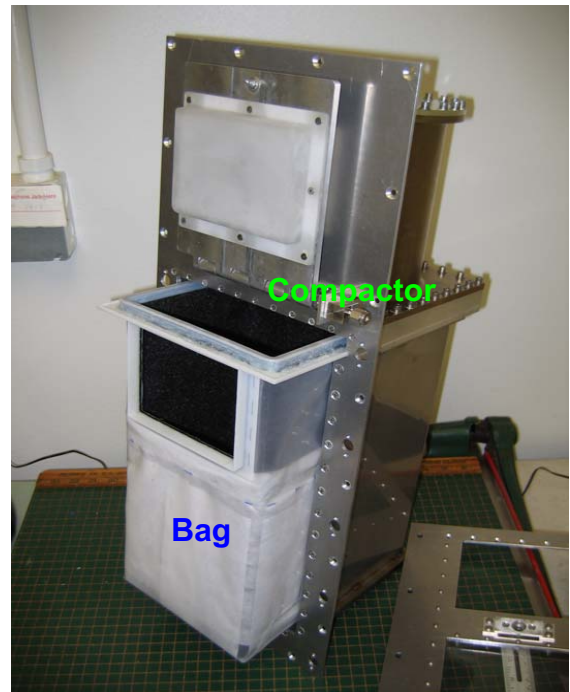
Figure 8. Wet Waste Containing Microgravity Compaction Bag.
