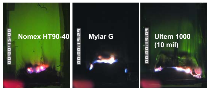
Figure 3: Front view pictures of microgravity flames on three different fuels samples at the ULOI. The concurrent forced flow velocity was 30 cm/s. The red LED in lower left is the same true brightness, giving an indication of the relative brightness between the flames. The green LED was not used for the Mylar as it caused too much specular reflection.
