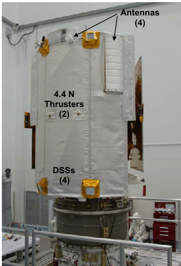
Figure 4. The MESSENGER spacecraft 2 weeks before launch. Highlighted here are the ceramic-cloth sunshade, the four DSSs with attenuating filters, the phased arrays and low-gain antennas under high-temperature radomes, and the 4.4-N pro-Sun thrusters.
