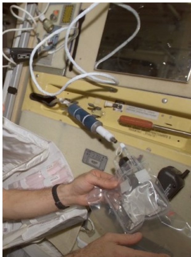
Figure 3. SVO-ZV Flush Water Sample Collection
