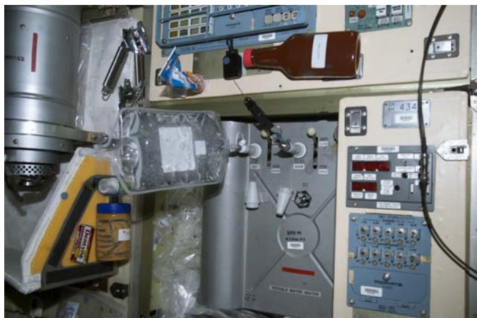
Figure 2. SRV-K Galley Located in Service Module
