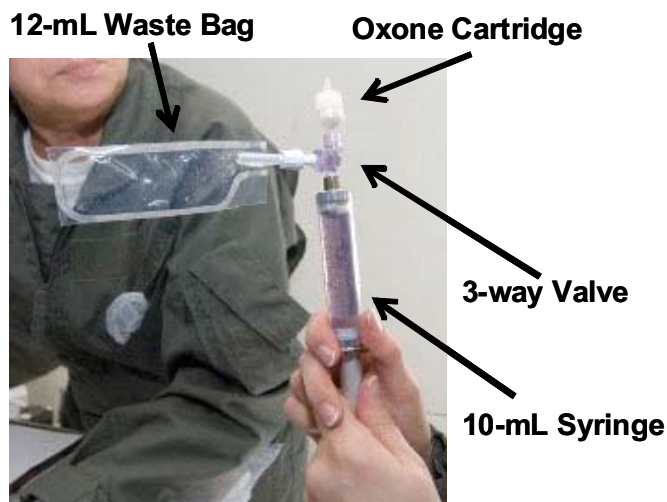
Figure 1. Photograph of the 3-way valve in flight. Syringe has been filled through the Oxone cartridge and the sample bag removed.
