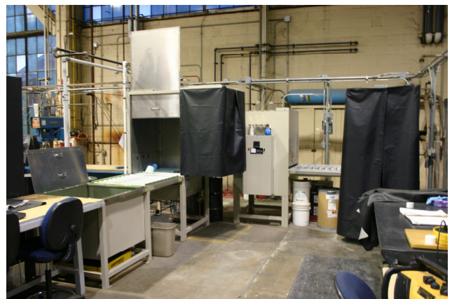
Figure 38 – Fluorescent Liquid Penetrant Inspection Line
