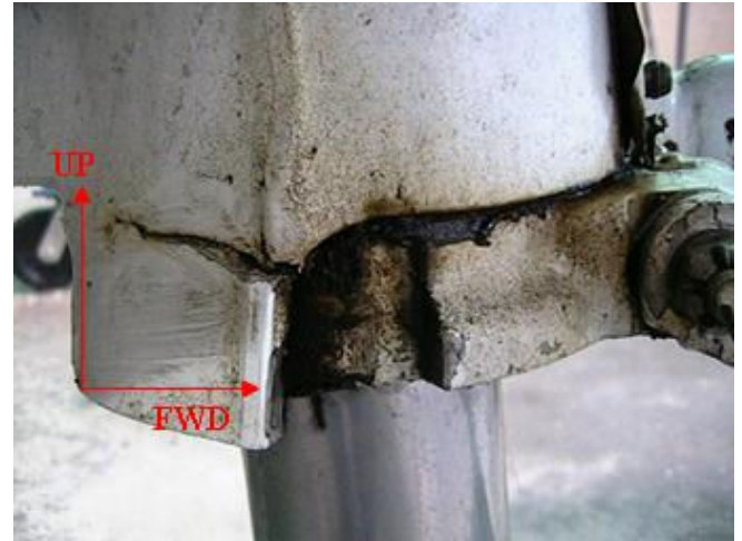
Figure 29 – Crack in Nose Gear Oleo Strut Housing (Piper Navajo)
