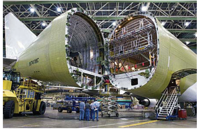
Figure 2 – First Swing Tail Opening [3]
