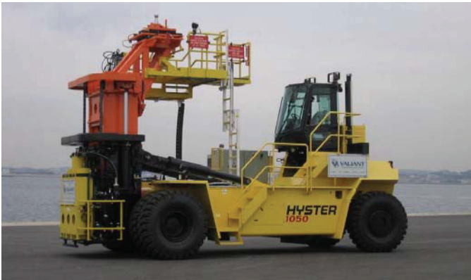
Figure 3 – Mobile Tail Support
