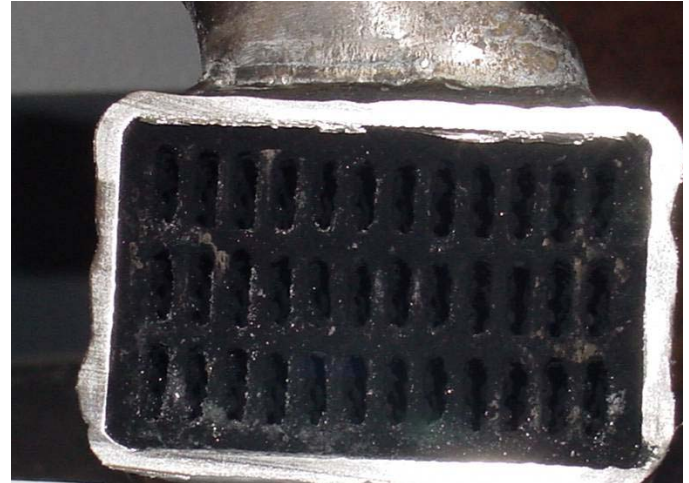
Figure 12 Deposits at EGR cooler inlet following 200 hour engine fouling test (2).
