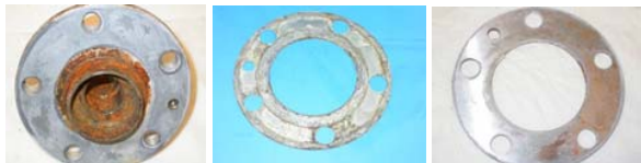
Fig. 04 / Hot-dip zinc galvanized steel shield, carbon steel / shield / HBU inner ring were bolted together, salt spray test ASTM B117
