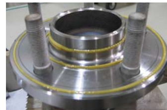
Fig. 01/ Molykote paste beads on the flange
