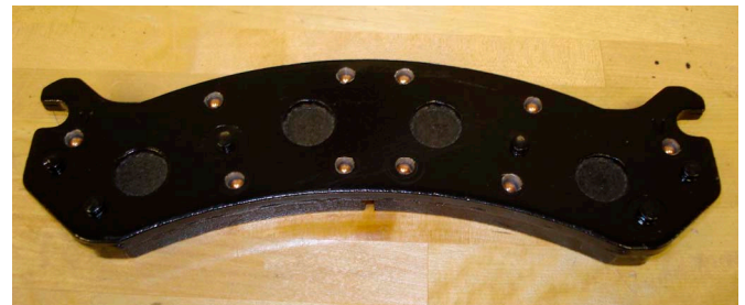
Figure 4: Brake-Pad with Vibro-Impact Dampers in strategically located holes in the backing plate.
