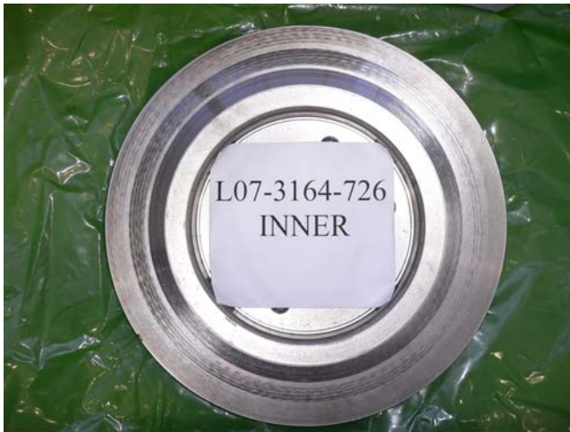
Figure 4: Post-test Inner Rotor Face Example
