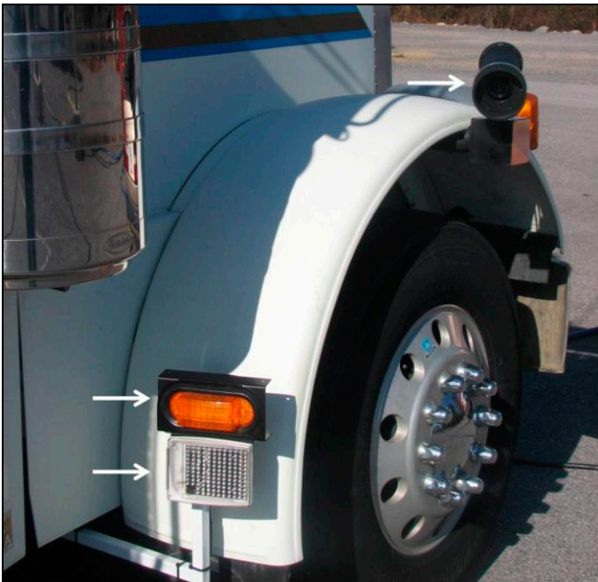
Figure 3. Camera and Illuminators mounted at the tractor passenger-side front fender.
