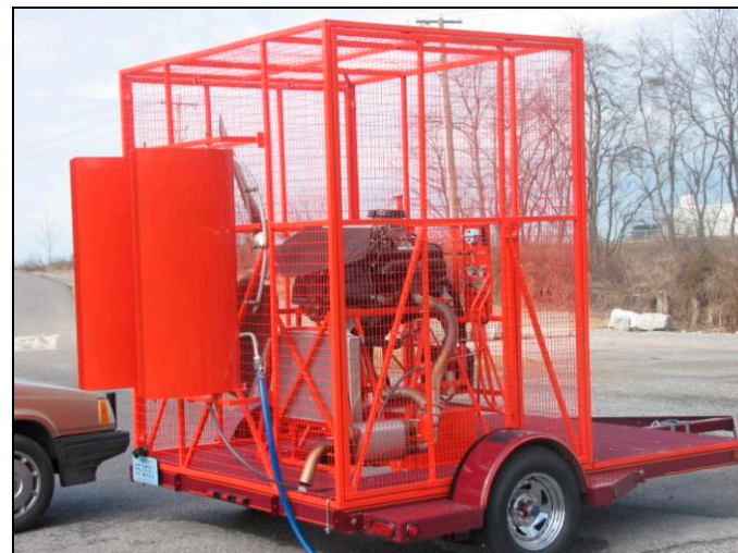
Figure 5. Wind/spray generation system.
