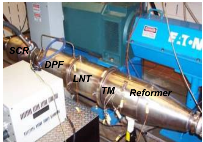
Figure 5: System Configuration (Reformer Inlet to SCR Out)
