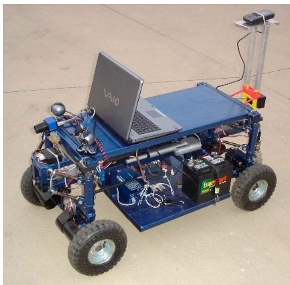
Figure 3: Mini ODY-ERA (mOE), custom-made 1:3 scale autonomous vehicle.
