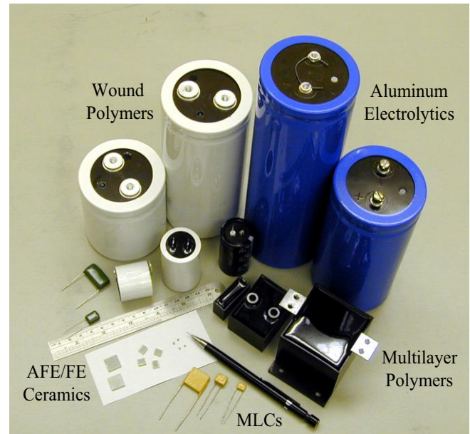
Figure 2. Photograph showing the major capacitor types produced for medium power inverter applications. The aluminum electrolytic capacitors are in the 5,000 to 10,000 \mu F 450 V range, The wound polymer capacitors are in the 250 \mu F 600 V range, the multilayer polymer capacitor compounds are in the 3 \mu F 600 V range. The largest multilayer ceramic capacitor shown is a 1 \mu F 500 V rated capacitor, and the ant ferroelectric/ferroelectric capacitors are 5 \mu F 250 V range.
