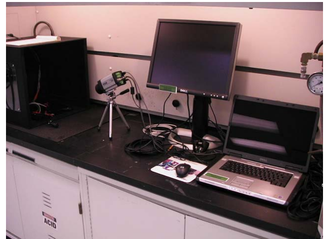
Figure 2. FLIR Systems ThermoVision® A20M Infrared Camera Set-up.
