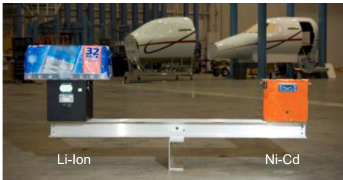
Figure 1 – Weight comparison, Li-Ion vs. Ni-Cd [31]
