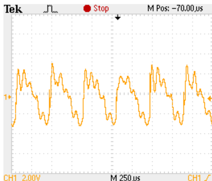
Figure 1: DC Ripple Voltage of Early 6-Pulse TRU
