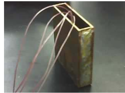
Figure 5. An integrated leak-proof TES column with side plates soldered and thermocouple wires instrumented
