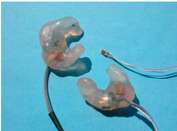
Figure 4. Indy Racing League type earplugs made by Sensaphonics using three Delphi (AD 193) linear sensors in an orthogonal array used by AFRL subjects in a research program reported in Knox et.al. 2004. Also pictured is the new Endevco 7273GT tri-axial sensor made for studies of head acceleration – small enough to be placed in the ear canal portion of the earplug
