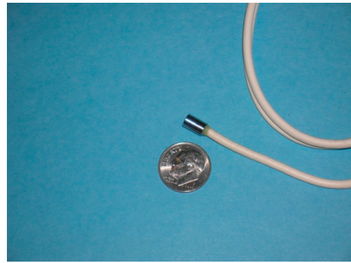
Figure 5. The Endevco 73M1 tri-axial accelerometer with a +/-, 6K g range and resonant frequency of 180K Hz was made for AFRL for testing at the University of Virginia in a study led by Dr. Bass. It is small enough to fit in the ear canal though not as small and light as the 7273GT.
