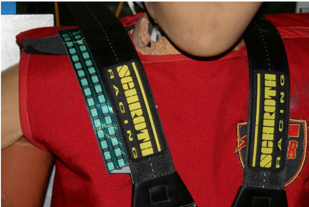
Figure 4. Tekscan Grid in Place Under 2-inch (50 mm) Belt on THOR ATD
