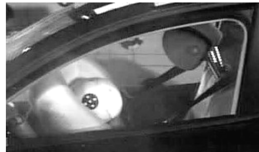
Figure 1: Limited optical observation during a crash test complicates motion analysis of the dummy head
