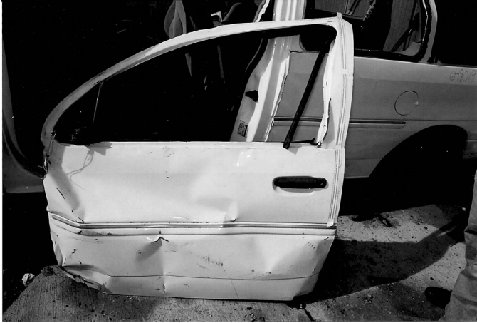
Figure 2. Door suffered relatively little damage in spite of being torn from hinges.
