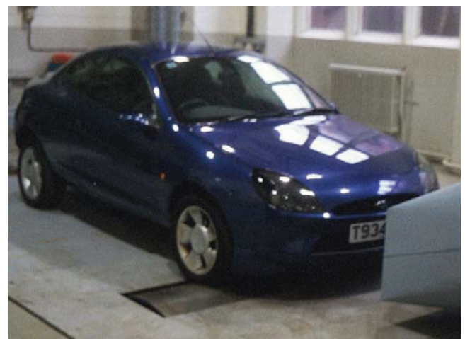
Fig. 1 Chassis dynamometer with test vehicle.
