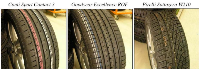
Figure 3: The tire variants used (dimension 225/45 R17)
