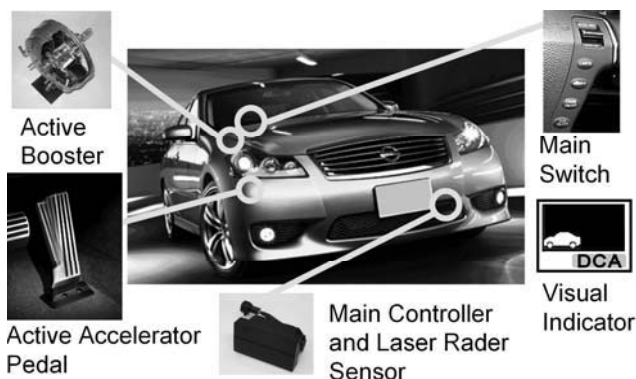
Figure 1 Main Components of the DCA
