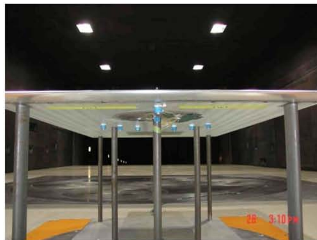
Figure 8. The plastic collar and screw underneath the table to secure the flush mount microphones.
