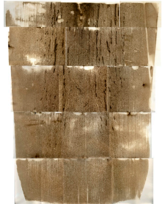
Figure 1. Sulfur-print of an up-hill teemed ingot.
