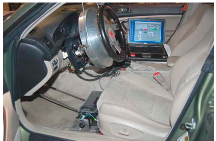
Figure 1: BTR Mounted in Vehicle (with ASC also Shown Mounted in Vehicle)
