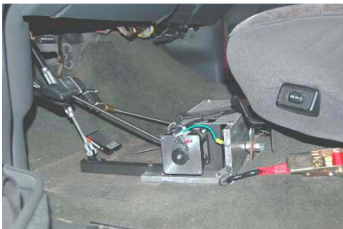
Figure 2: Close-up View of BTR Mounted in Vehicle
