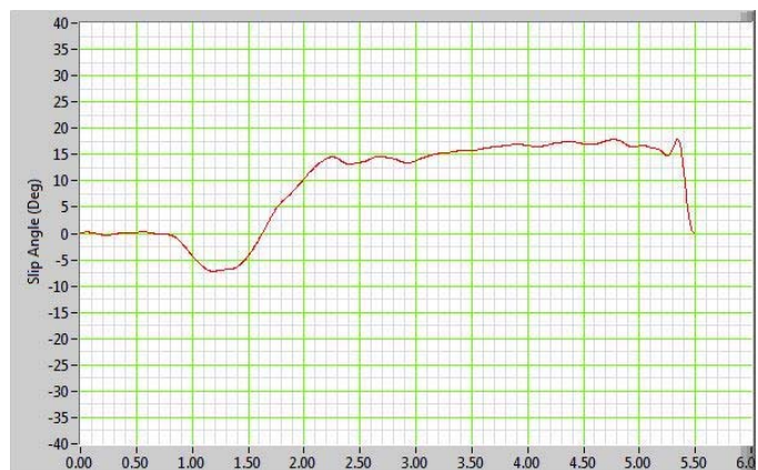
Figure 12. Typical slip angle trace when the test vehicle does not spinout or pass the NHTSA yaw rate criteria
