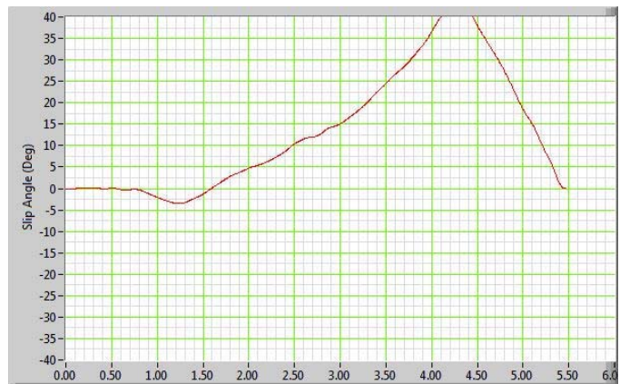
Figure 11. Typical slip angle trace when the test vehicle has a classic spinout response
