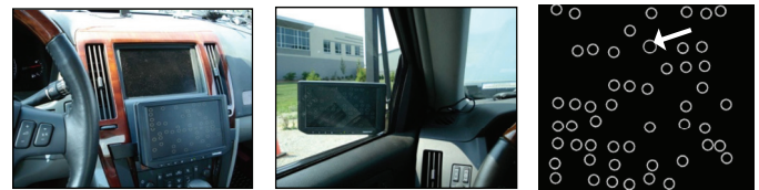
Figure 5. Center console (shown on left) and left side mirror (shown in the middle) visual distraction task locations. A sample visual distraction task stimulus (derived from the Surrogate Reference Task or SuRT) is shown on right. Drivers were required to verbally indicate which half of the screen contained a larger circle (indicated here with an arrow).
