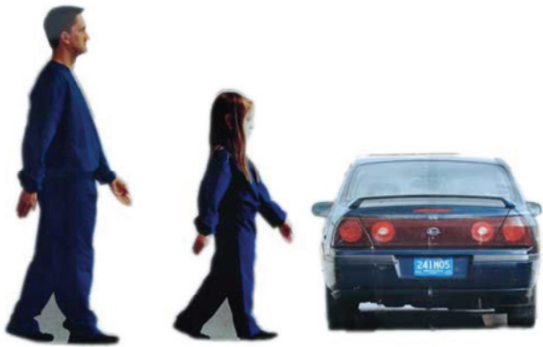
Figure 2. The full-scale adult (male) pedestrian, child (female) pedestrian, and vehicle pop-up targets used to create scene changes. (For clarity, targets are not shown to scale).
