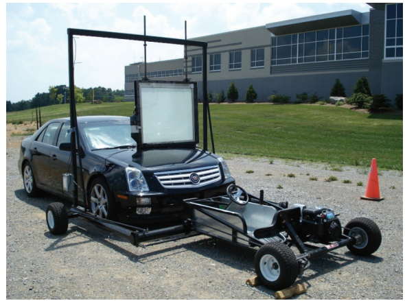
Figure 1. The position of the visual occlusion window device in front of the test vehicle.
