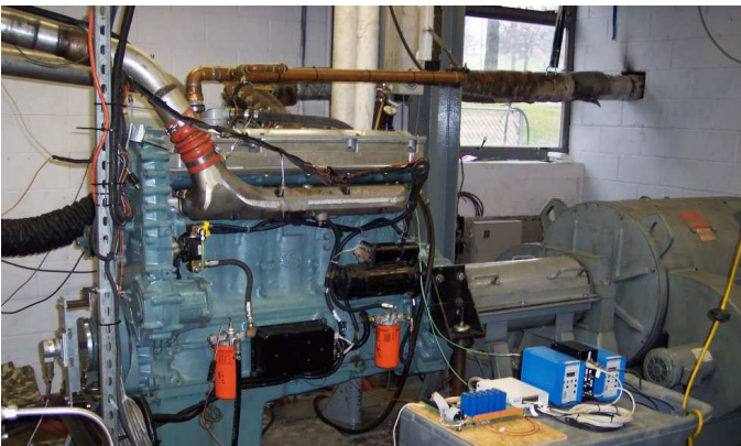
Figure 1 WVU Test Cell with 1992 Detroit Diesel Series 60 Engine Mounted
